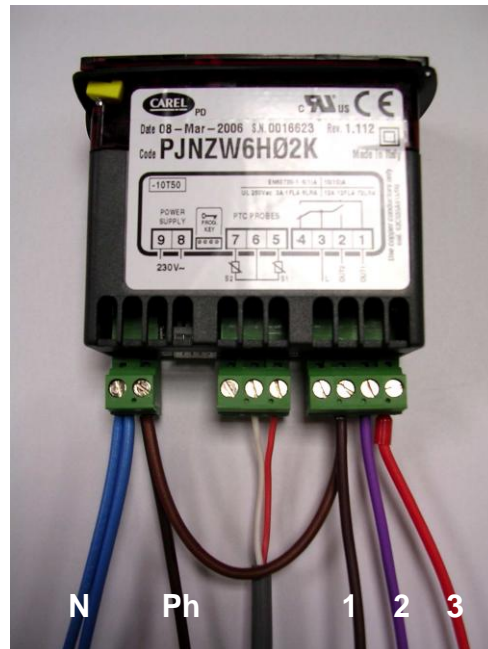
Thermostat CAREL (W6020.1) câblage existant
